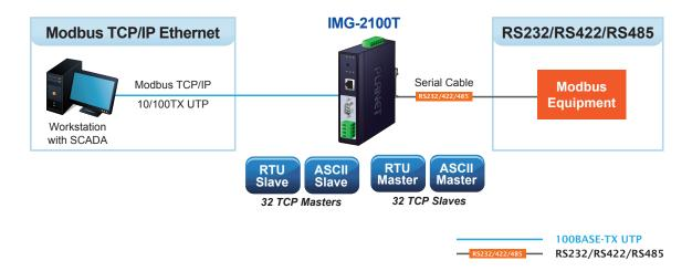
The advantage of having the IMG-210XT is to assist users to build an industrial environment between the Modbus TCP/IP Protocol and the Modbus RTU/ASCII Protocol easily, thus offering an application solution to the industrial control equipment without Ethernet ports and the industrial control equipment can only control through an industrial PC workstation or industrial control panel.
